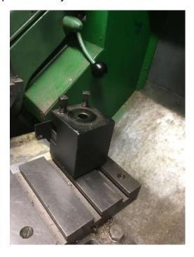
The first action is to remove 1" from the base of the holder, mill a T-slot and fit T-nuts to locate in the Myford Cross Slide
