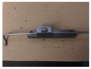
The Pointer aligns with markings on barrel adjusted by loosening the knurled screw
