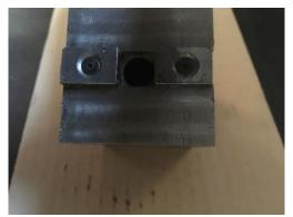
Now with a piece of steel make a 1" thick sub plate in which you mill the Myford keyway slot
